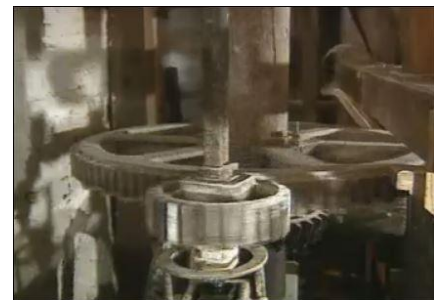
Transmitting the Water to the Millstone
